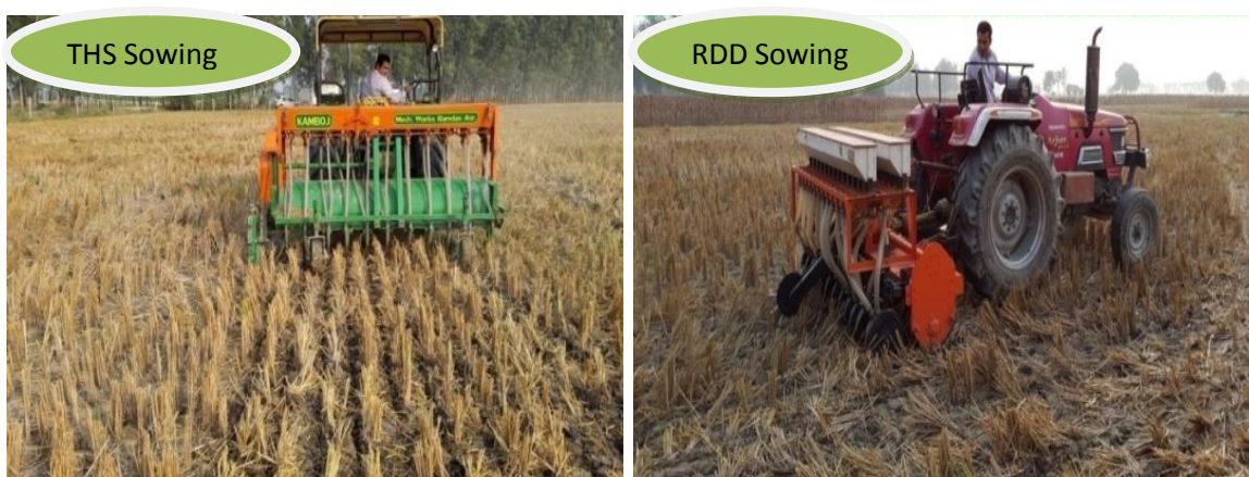
Plate 3. Wheat seeding in rice residue using Turbo Happy Seeder (THS) and Rotary Disc Drill (RDD) at Village Taraori (Karnal)
